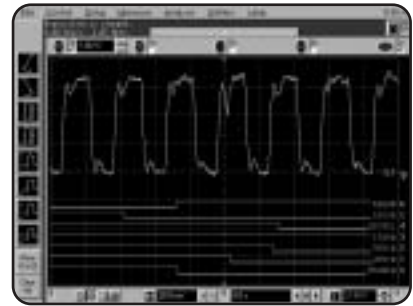
Figure 3. Address-dependent coupling can be seen interfering with the clock signal in this PCI bus-based system.
